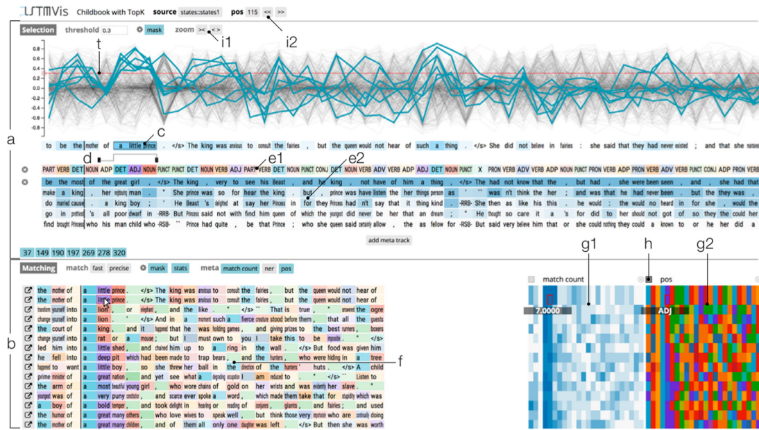
Fig. 12. LSTMVis tool [98] showing the activations of the hidden states in a RNN model for a sequence of input units chosen by the designer. When the designer chooses a text range, the visualization displays how hidden state values changed through the processing of such text range (a). The visualization provides several interactive tools, such as the capability of choosing a threshold for highlighted hidden states (t), the matching and comparison of input sequences resulting in similar hidden states (b), and the visualization of user-defined meta-data about the model (g1, g2).
