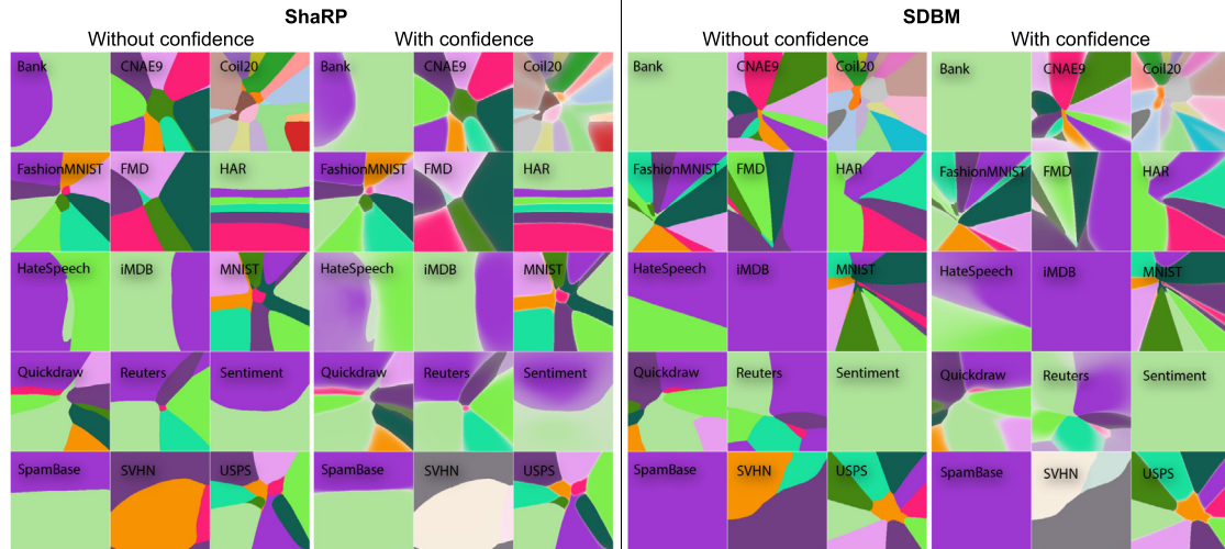
Fig. 13. DBMs created by ShaRP and SDBM for all studied datasets, visualized without and with saturation-encoded confidence. The classifier is frozen per dataset. Immediately noticeable are the 2-class cases where SDBM produces degenerate DBMs (Sentiment, SpamBase datasets). We also see SSNP’s starburst pattern leaking into SDBM (FashionMNIST, MNIST datasets), which ShaRP avoids.
