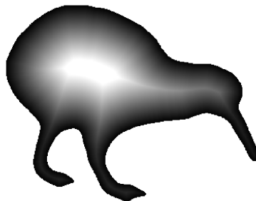
Figure 1: The distance transform of an object. The pixel intensity denotes distance to the object boundary.
