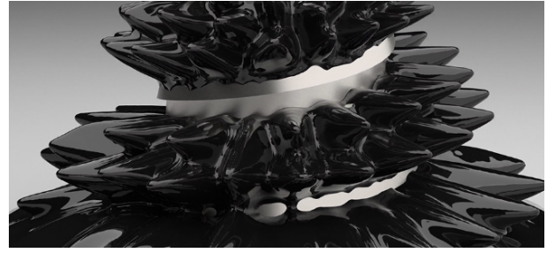
Fig. 48 A ferrofluid climbs up a steel helix under a strong external upward magnetic field to create surface spikes [305].
