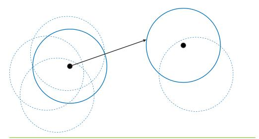
**Figure 7-8.** The Dispersion of Particles The black dots are surface particles, and the circles represent their influence areas. Dashed circles are neighboring particles' influence areas. On the left is surface particle x, with its density higher than surface particle y on the right. Therefore x might move to the edge of y's influence area.
