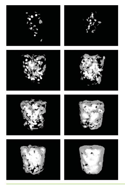
**Figure 7-9.** The Distribution Methods at Work: Surface Particles Spread over a Group of Fluid Atoms in the Form of a Cylinder
