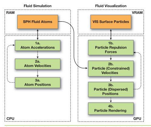
**Figure 7-2.** The Fluid Simulation Loop Performed on the CPU Together with the Fluid Visualization Loop Performed on the GPU
