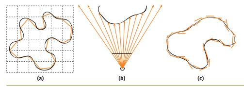
**Figure 7-1.** Methods of Visualizing Implicit Surfaces *(a) Marching cubes, (b) ray tracing, and (c) the point-based method.*
