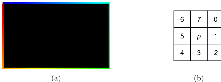
Figure 3.6: (a) Initial boundary labels, (b) numbering scheme for pixels adjacent to p .
