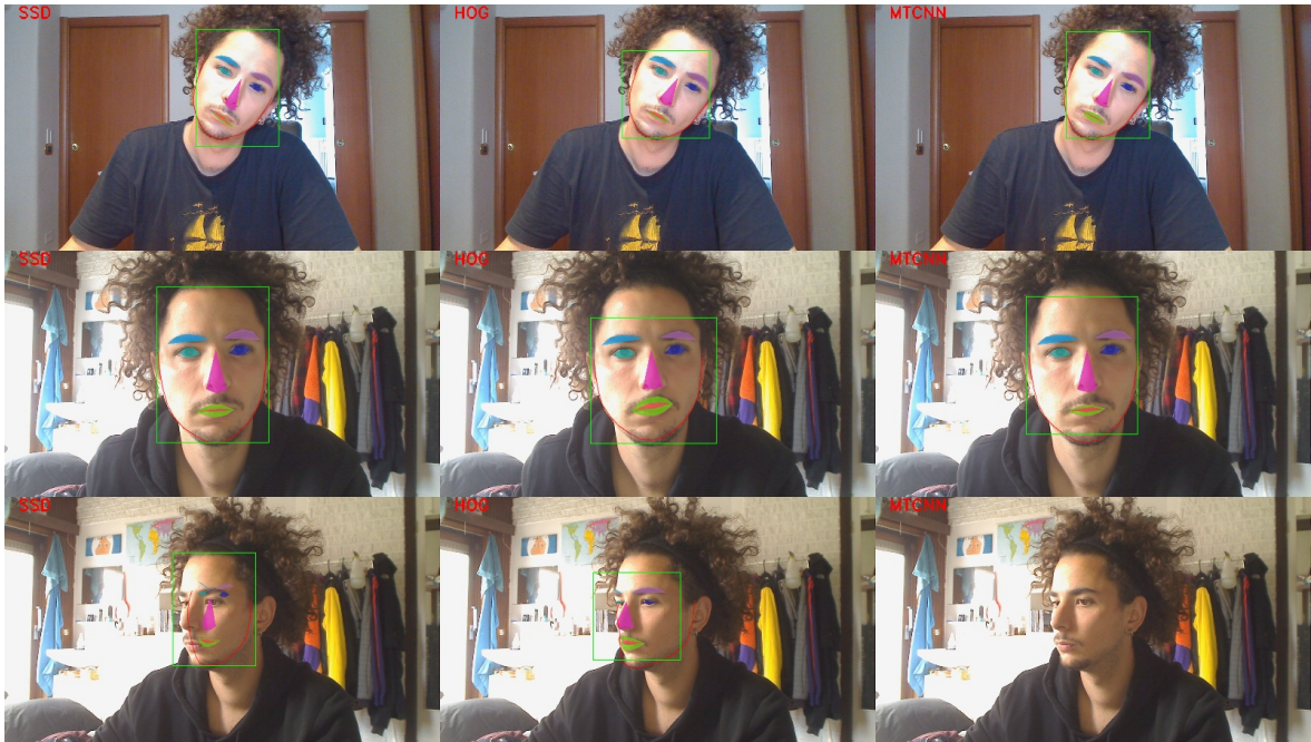
Figure 4.2: A visual representation of how the three face detectors set basis for landmarks positioning. An interpolation has been performed between landmarks, so to see the area they are supposed to refer to.
