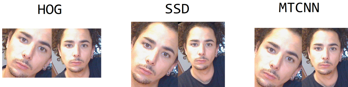
Figure 4.4: A visual comparison of how the alignment is performed given that the landmarks are set on the basis of each face detector considered.
