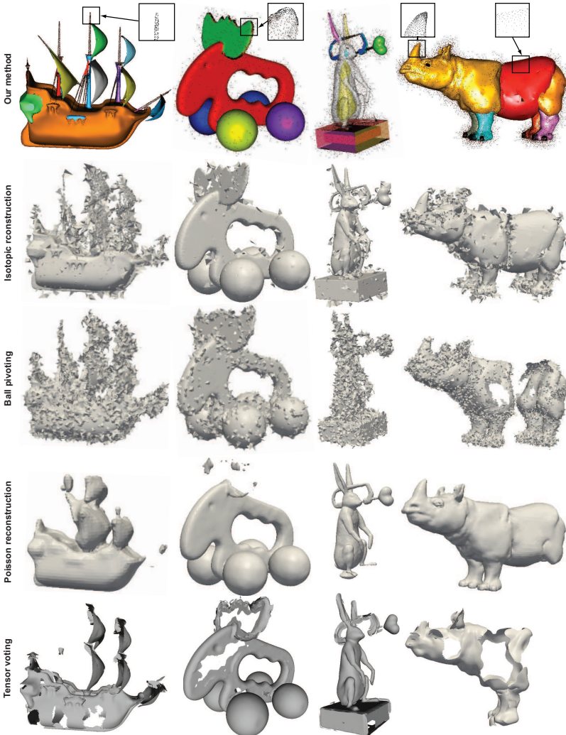
Figure 4.9: Shape reconstruction comparison for noisy point clouds with intersecting manifolds. From top to bottom, rows: our method, isotropic reconstruction [39], ball pivoting [12], Poisson reconstruction [77], and tensor voting [105]. Zoom-ins show point cloud details of selected model areas, for getting insight into the sampling distribution.
