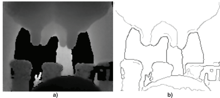
Figure 5.6: Depth image based detection of teats. Depth image (a) and its edges (b). See Sec. 5.4.1.2.
