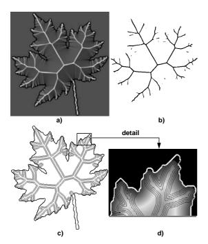
**Figure 9:** Singularity detector (a), skeleton neighborhood (b), inflated skeleton and original boundary (c), reconstruction detail (d)
