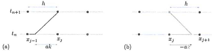
Figure 13.2: Tracing the characteristic of the advection equation back in time from the point (x_j, t_{n+1}) to compute the solution according to (13.29). Interpolating the value at this point from neighboring grid values gives the upwind method (for linear interpolation) or the Lax-Wendroff or Beam-Warming methods (quadratic interpolation). (a) shows the case a > 0 , (b) shows the case a < 0 .
