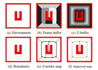
Fig. 1. Construction of the corridor map.
