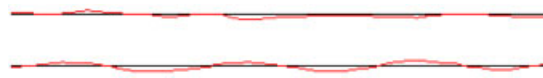
Figure 10. Two resulting pelvis trajectories (red) for the query paths (black). As can be clearly seen, the Gaussian smoothing path abstraction (below) preserves the natural oscillation of the pelvis whereas the standard method (top) does not.
