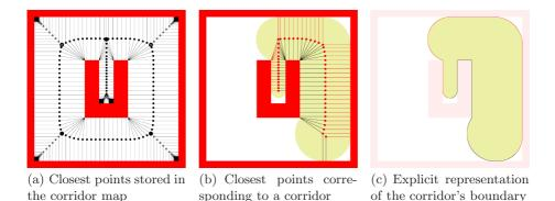
**Fig. 4.** Closest points to the obstacles. By concatenating the points with line segments and circular arcs, we obtain an explicit representation of the corridor's boundary.
