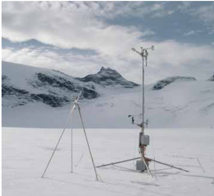
Figure 1. The automatic weather station at Storbreen, Norway. Measurements of humidity, temperature and wind are done at two levels, about 2 m and 6 m above the ice surface. The free standing sonic ranger (to the left) measures ice melt and snow accumulation. Photo: Liss M. Andreassen.
