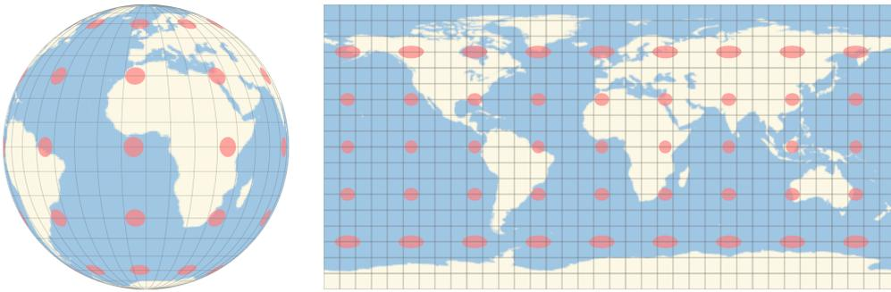
Figure 6: According to Gauss 'remarkable' theorem, it is impossible to make global map which preserves length and area. The pink disks are in both images the same. As you can see, this global map is distorted.
