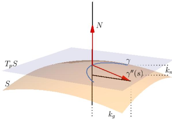
Figure 11: A graphical illustration of the construction of the geodesic curvature  $k_g$
