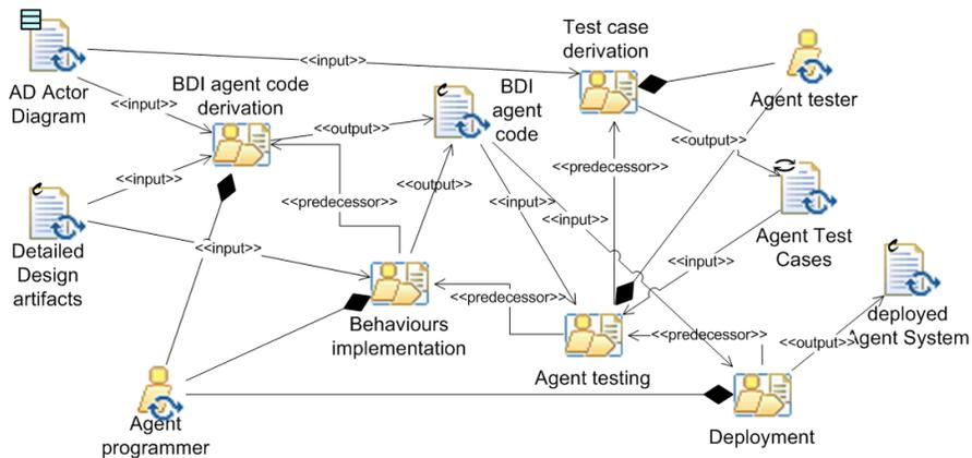
**Fig. 21** SPEM model showing the structure of the Implementation and Testing phase with in- and output work products. The phase takes in input the AD actor diagram and the outputs of the DD phase.
