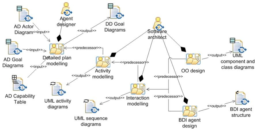
**Fig. 18** The structure of the Detailed Design phase described in terms of activities, involved roles and work products. Please note that the internal use of work products in output of an activity as inputs of the subsequent activities is not shown explicitly, to keep the diagram concise.
