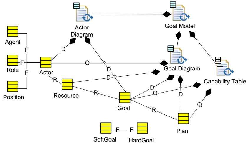
**Fig. 8** General structure of a *Goal Model*, composed of actor- and goal diagrams and the capability table, in relation to the meta-model elements, as used in the early and late requirements analysis phases and in the architectural and detailed design phases (D: define, R: relate, F: refine, Q: query).
