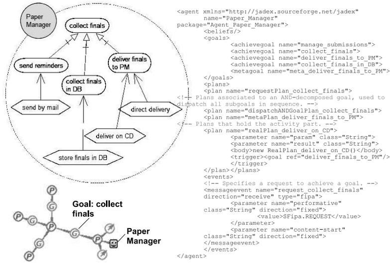
**Fig. 22** Left: Simplified goal diagram for PaperManager modelled using the *TAOM4e* tool. Right: part of the *Jadex* XML code generated with the *t2x* tool. Bottom: example *Jadex* run-time agent instance with activated goals and plans, visualized with the *Introspector* tool provided by the *Jadex* platform.
