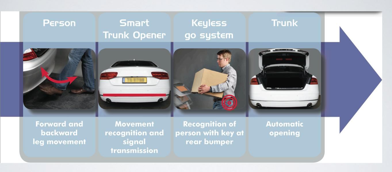
STO Provides automatic and hands-free access to a vehicle's trunk (based on a keyless entry system)
