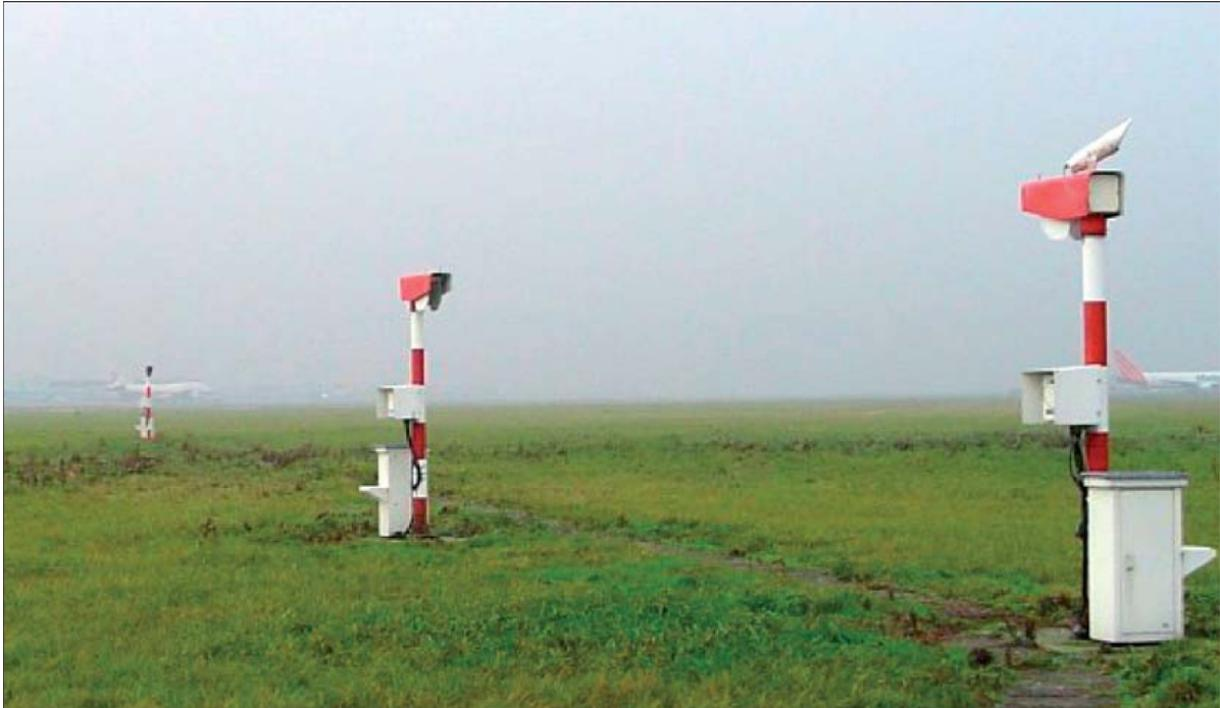
**Fig. 9.** A transmissometer set up located at Schiphol, the Netherlands. Right: projector and background luminance meter; Left: two light receivers. Source: *KNMI, 2005*.
