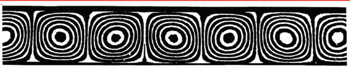
Figure 3. Side-view (differential interferograms) of two-dimensional convection cells in silicone oil in a rectangular box of relative dimensions 10:4:1, which is heated from below. Uniform heating produces convection “rolls” parallel to the shorter side (Van Dyke, 1982). The flow pattern is remarkable orderly!
