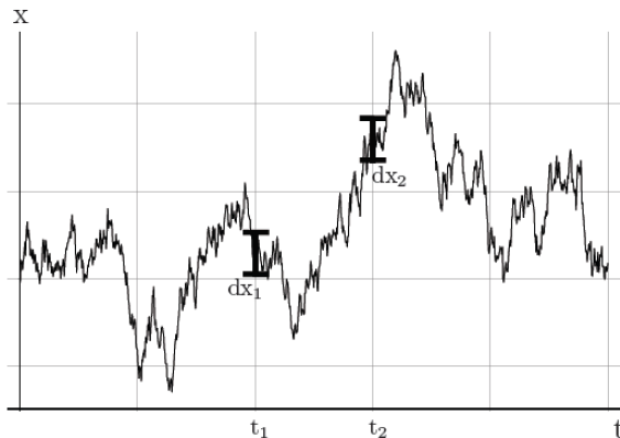
FIGURE 4. Sketch of the meaning of the joint probability function p(x_1, t_1; x_2, t_2) .
