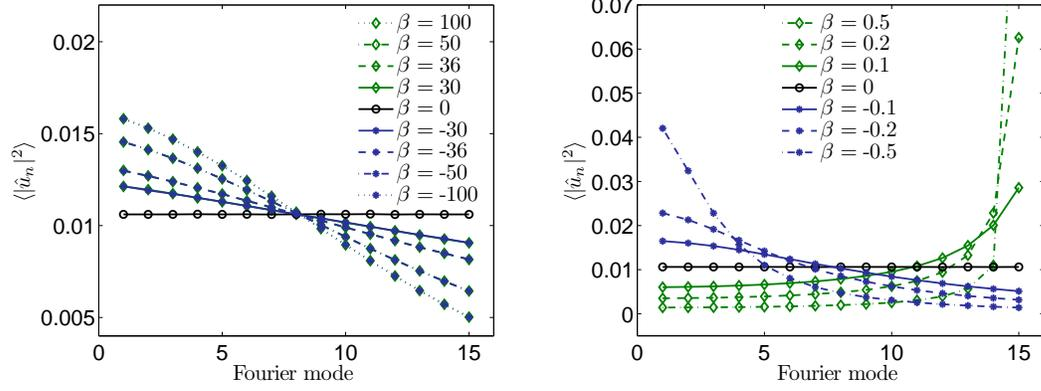
Figure 2: Mean kinetic energy spectrum, for different values of  $\beta$ . Left: BH equation. Right: KdV equation.
