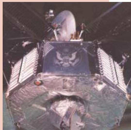
Side-view of Mariner IV clearly showing the TV camera underneath the octagonal structure. The 'Venetian blinds' on the sides were used for internal temperature control.
