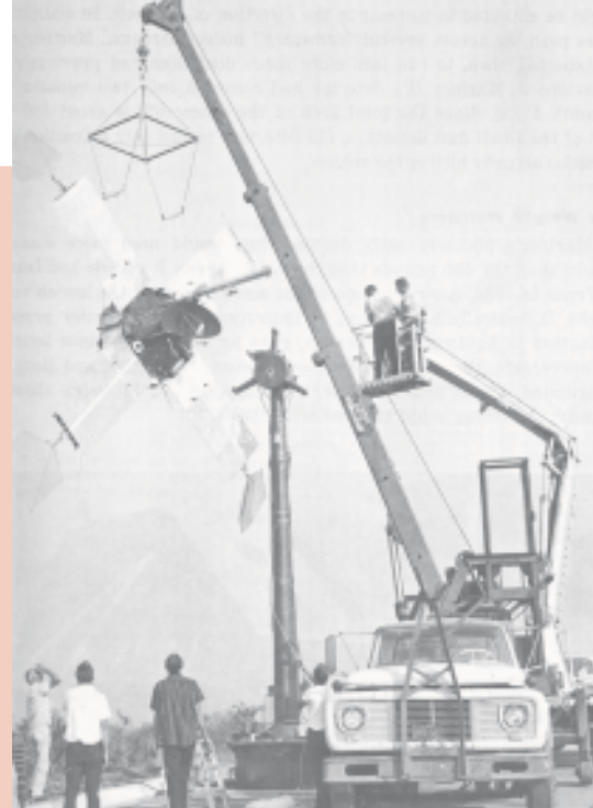
Radio-tests on the Mariner IV spacecraft. Compare the size of the craft against the JPL-engineers. Photos: NASA/JPL
