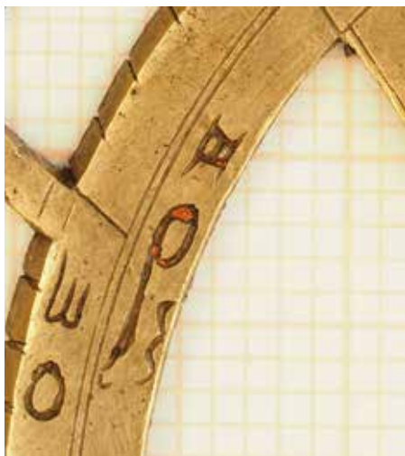
Fig. 3 Close-up of the engraving on the rete showing traces of red infill in the engraving. Note also the abbreviation of Aquarius.
