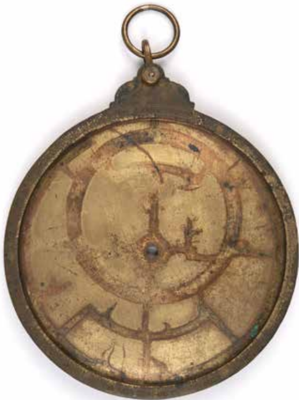
Fig. 2 (left) The mater of the Zuylenburgh astrolabe showing the ghost image of the rete with, (centre) a close-up of the throne and (right) side view showing the laminar construction.
