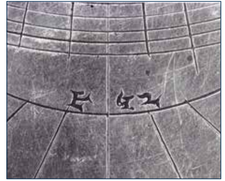
Fig. 10 (left) Detail from the plate for 52° from the Zuylenburgh astrolabe compared with (centre) the engraved latitude from AST0590 (authors' photo) and (right) #4516 (Milan) taken from Tomba & Brusa, p. 38.
