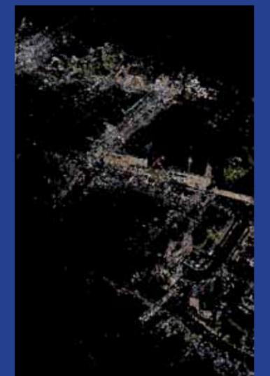
Lidar and sparse point clouds. The panoramas are fitted by aligning these point clouds.
