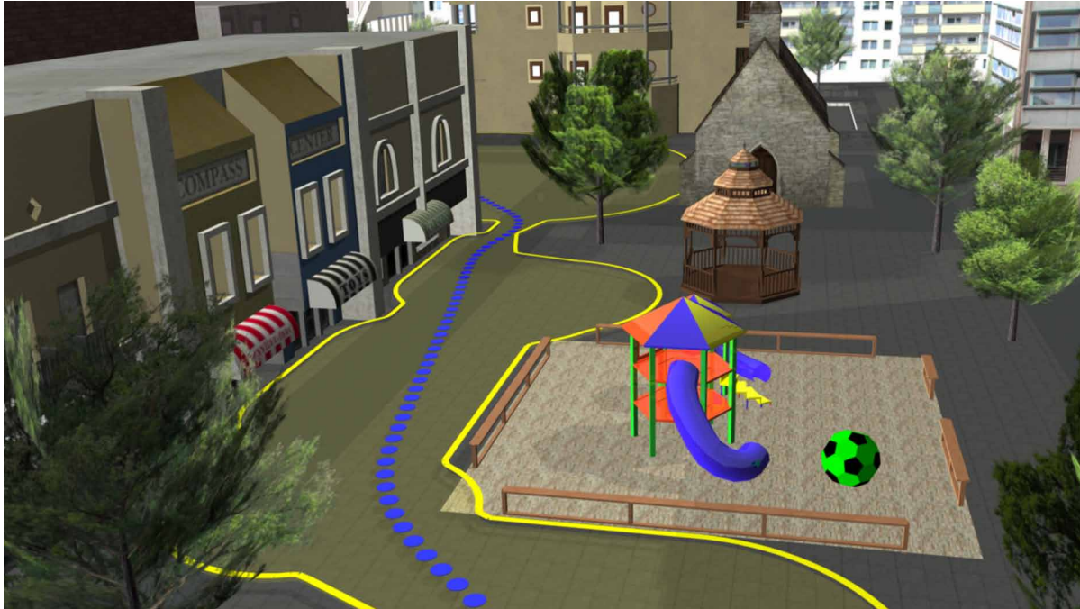
Figure 10. A smooth path computed by the Indicative Route Method using the Explicit Corridor Map (Geraerts, 2010)
