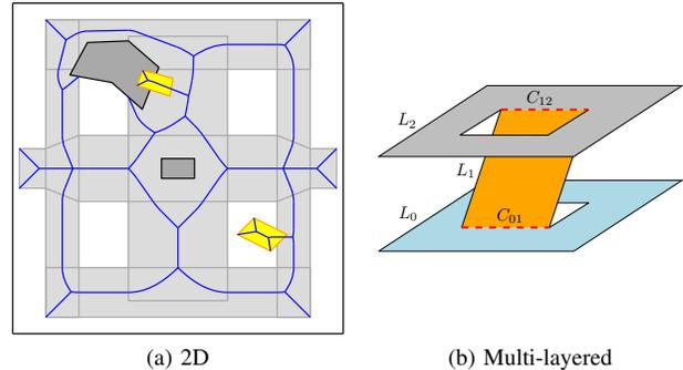
Fig. 5. Constructing an environment. (a) Users can define the walkable space of a layer in terms of walkable areas (light gray), obstacles (dark gray), and openings (yellow). The medial axis of the combined walkable space is shown in blue. (b) Multi-layered environments consist of 2D layers  $L_i$  and connections  $C_{ij}$ . The layers are drawn in different colors for clarity.
