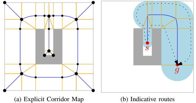
Fig. 4. A simple environment with obstacles (shown in gray). (a) The ECM is the medial axis (blue) annotated with closest-obstacle information (orange). This subdivides the walkable space into polygonal regions. (b) A path along the medial axis induces a corridor (light blue) due to the ECM’s annotations. Within the corridor, we can define any indicative route from  $s$  to  $g$ ; two examples are shown in black.
