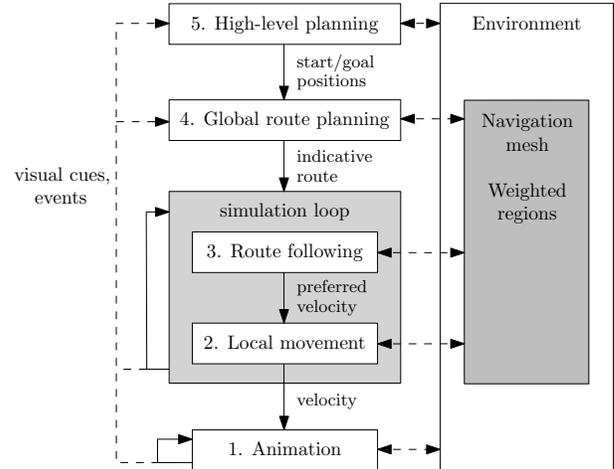
Fig. 1. A five-level hierarchy for path planning and crowd simulation systems. The geometric levels, which can be solved using our algorithms and software, require an efficient *navigation mesh* of the environment.
