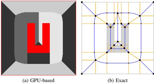
Fig. 6. Two ways to generate the ECM. (a) Using rendering techniques, we can approximate the Voronoi diagram on the GPU frame buffer. (b) External libraries such as Boost and Vroni can compute the Voronoi diagram, which we convert to an ECM. Graph elements inside obstacles are filtered out in a post-processing step.
