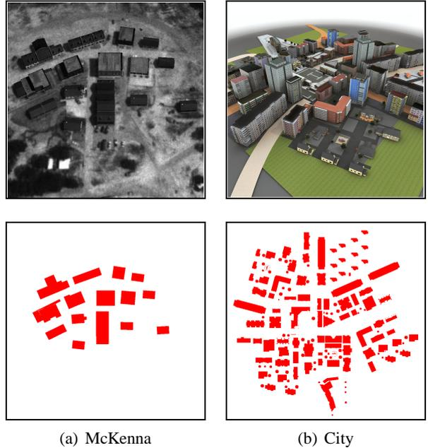
**Fig. 2.** The two test environments. The first row shows the 3D models and the second row the corresponding footprints, used for constructing the corridor maps.
