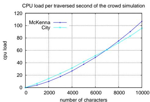
**Fig. 4.** The relation between the number of characters and the CPU-load per second traversed time.
