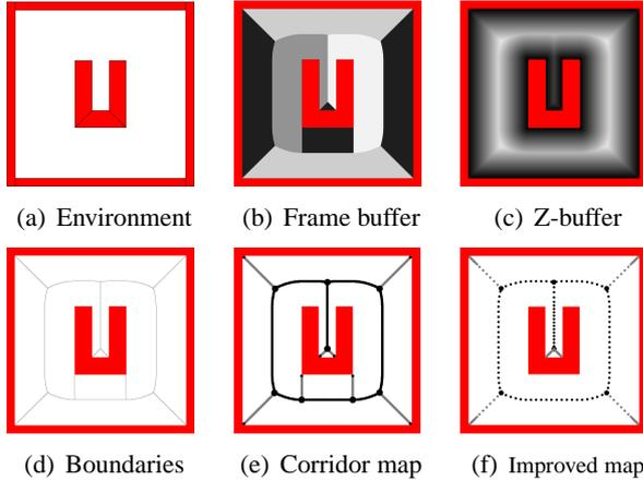
**Fig. 1.** Construction of the corridor map.
