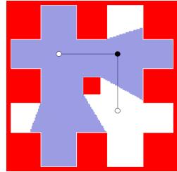
Fig. 1. The coverage and maximal connectivity criteria have been met: the reachability regions of the white vertices cover the free space and are connected via the black vertex.
