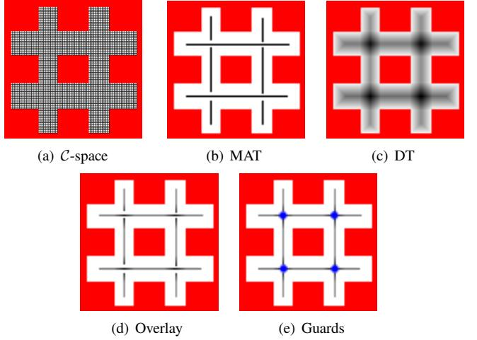
Fig. 2. The creation of candidate guards. Figure (a) shows the free (white) cells of the discretized  $\mathcal{C}$ -space of Figure 1. Figure (b) shows the cells of medial axis transform and (c) the distance transform. Dark cells correspond to a large distance to the closest obstacle while light cells correspond to a small distance. In (d), the overlay of the MAT and DT is shown. Finally, (e) shows the four guards having the largest distance in the overlay.
