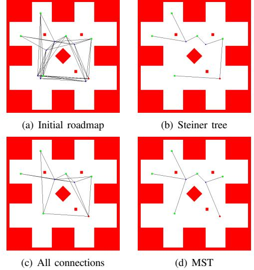
Fig. 4. Roadmap pruning. Figure (a) shows (among other roadmap elements) the connectors (small spheres) that lie in the overlapping regions. From this roadmap, an approximated shortest roadmap is calculated in (b). In (c), all collision-free connections are added. Finally, (d) shows the minimal spanning tree (MST) of the roadmap in (c).
