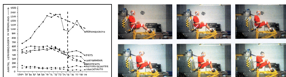
Figure 5 – Two pictures from the PLON unit Traffic and Safety : the number of traffic casualties over the years (left), and the motion of the car driver’s body when wearing a safety belt (right). The physics involved is summarised by the (empirical) equation F \cdot s = \frac{1}{2} \cdot m \cdot v^2 : given a certain initial speed v , the safety belt lengthens the displacement s of the body and thus reduces the force F exerted on the body during a collision. The 1975 marker and trends (dotted lines) have been inserted by the author.
