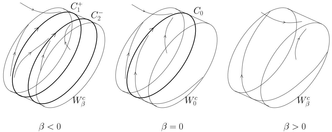
Collision and disappearance of two limit cycles:  $C_1^- + C_2^+ \rightarrow \emptyset$
