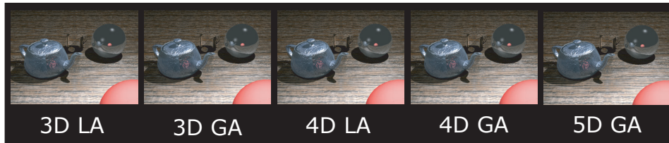
Figure 1: The same result can be achieved in many ways. These images are identical, but each one was rendered using a different model of 3D Euclidean geometry. The scene consist of 5 objects modeled with about 7800 triangles: a textured/bumpmapped teapot, a transparent drinking glass, a reflective sphere, a red diffuse sphere, and a textured/bumpmapped piece of wood.
