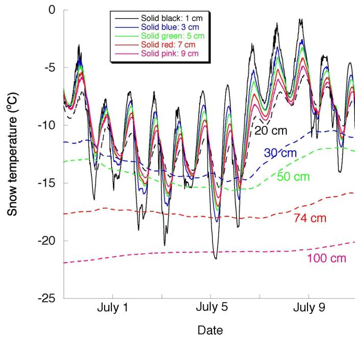
**Figure 2.9:** An excerpt of the snow temperature data between June 29 and July 11. The damping of amplitude and the phase lag with depth are clearly visible.
