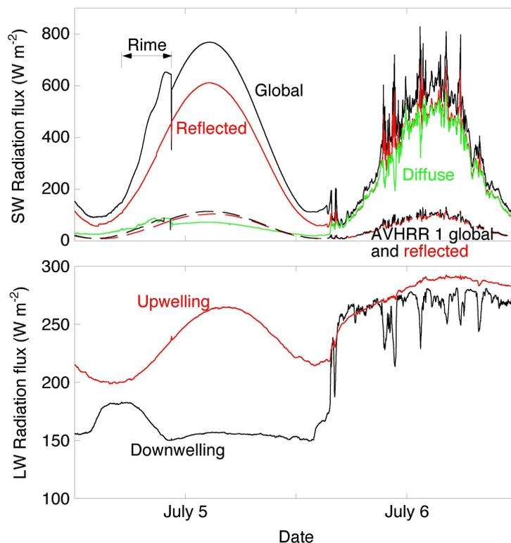
**Figure 2.4:** Shortwave (upper panel) and longwave (lower panel) radiation on a clear and an overcast day. Global, reflected and diffuse radiation are measured using Kipp en Zonen CM21, the AVHRR 1 global and reflected radiation are shown as an example of the narrowband measurements with 9 pairs of Kipp en Zonen CM11 sensors. Longwave radiation is measured using Kipp en Zonen CG4 sensors. Rime formation on the CM21 domes disturbs the SW measurements.
