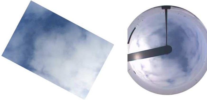
**Figure 2.7:** Two sky images taken at approximately the same time (17<sup>th</sup> of July, 19.14 UTC), using the sky camera with a fisheye lens (left) and the total sky imager (right). Cloud cover percentage can be calculated from the TSI images using a software package.
