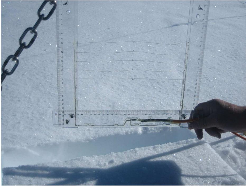
**Figure 2.8:** *Special thermocouple sensors were assembled at IMAU for measuring snow temperature in the first 10 cm of the snowpack.*
