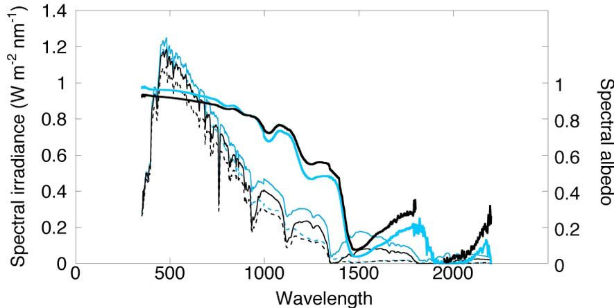
**Figure 2.6:** Spectral irradiance under clear (blue) and cloudy (black) conditions, as measured with the ASD Field Spec FR spectroradiometer. Thin solid lines are incoming radiation, dashed lines represent reflected radiation. Clear measurement taken at July 5<sup>th</sup>, 15.00UTC; cloudy measurement taken at July 7<sup>th</sup>, 15.00UTC. Spectral albedo is represented by the thick solid lines. These measurements have yet to be corrected.
