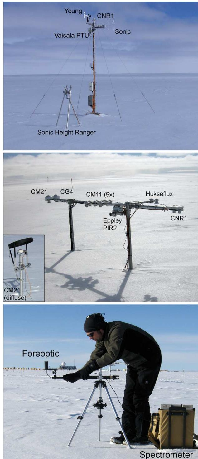
**Figure 2.3:** Top: The AWS (Young = wind monitor, CNR1 = shortwave and longwave radiation measurements, Vaisala PTU = temperature, pressure and humidity, Sonic = sonic anemometer); Middle: Radiation setup; Bottom: Spectroradiometer setup. See text and Appendix A for more information about the instruments.
