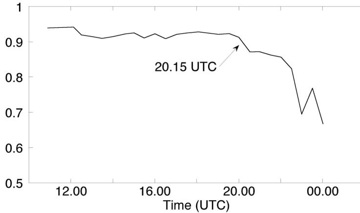
**Figure 2.5:** Ratio between integrated spectrometer hemispherical flux and the incoming flux measured by the CM21. During the day, the difference may be caused by a differing cosine response and by the different wavelength ranges of the spectrometer (350 - 2,200 nm) and the CM21 (300 - 3,000 nm). After 20.15UTC (18.15 local time), the poor cosine response of the ASD clearly shows up.
