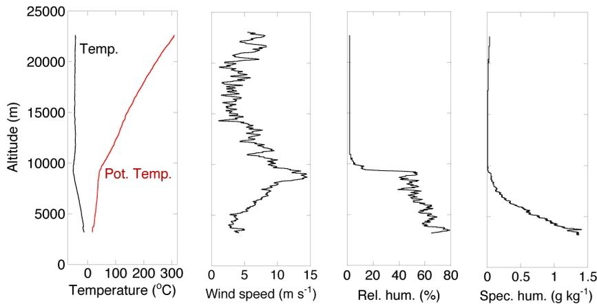
**Figure 2.10:** Typical vertical profiles of temperature, wind speed and relative humidity (measured), and potential temperature and specific humidity (calculated). Wind direction and pressure are also recorded but not plotted here. Data is from June 17<sup>th</sup>, 14.00UTC, a clear day.
