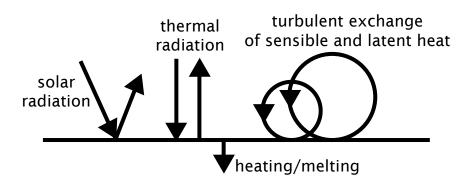
Solar and thermal radiation are the dominant terms in the energy balance over a flat snow surface.
