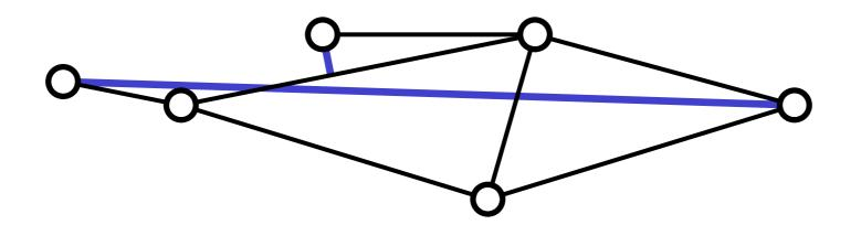
The *resolution* of a drawing is the ratio between the diameter and the shortest distance between two non-incident features of the drawing.
