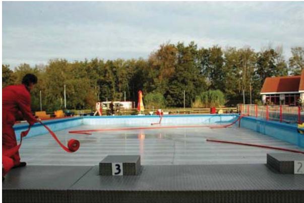
Figure 1: Fire brigade filling cold ( 17^{\circ}\text{C} ) swimming pool with warm ( 28^{\circ}\text{C} ) water from adjacent pool. After filling the floating 'blanket' is removed, leaving a sharp interface at a depth up to 40 cm.
