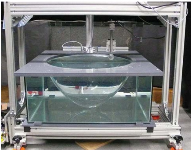
Fig. 1 Photograph of the experimental set-up. The paraboloidal tank is visible in the center of the larger rectangular outer tank. The oscillating sphere, that can be lowered into the fluid, is located above the tank to the right of the center, and the dot pattern on the light bank is behind the tank
