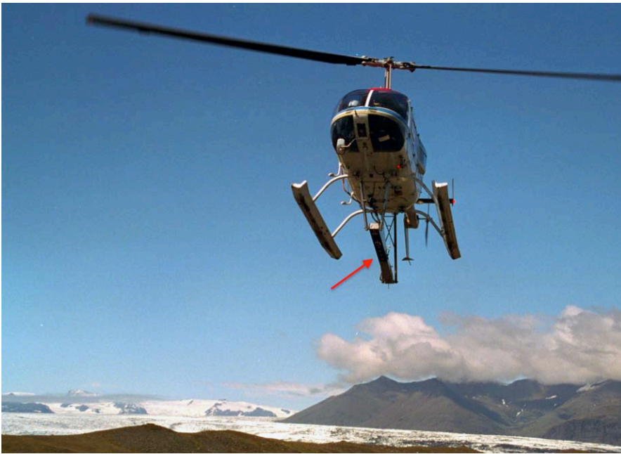
Figure 4.8. Field campaign on Iceland to measure band albedos. The instrument beam is indicated by the arrow. It has sensors to measure reflected radiation in the NOAA-AVHRR Channels 1 and 2, and in the Landsat TM bands 2 and 4.
