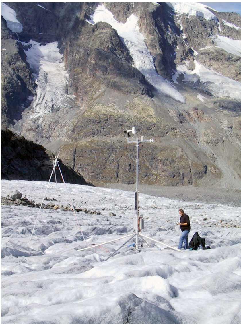
Figure 1.4. On a glacier with strong ablation, one should not anchor weather stations but let them stand freely on the ice surface. A construction with four legs attached to each other by steel cables performs well. The tripod with the sonic ranger is drilled into the ice, of course. We owe many smart ideas to technician Wim Boot, here working on the Vadret da Pers (September 2000).
