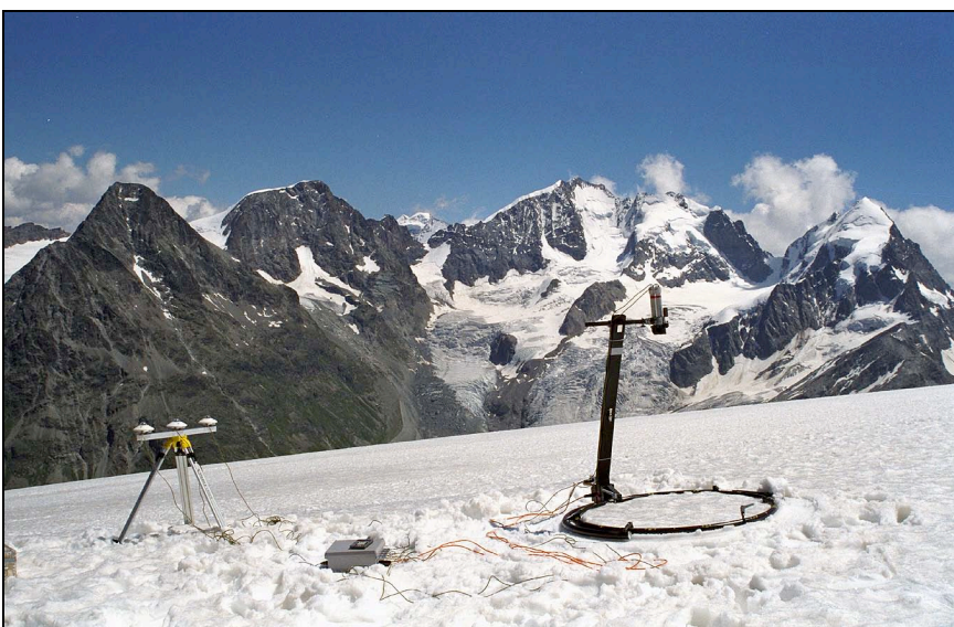
Figure 4.14. Studying the reflectance characteristics of firn in the accumulation zone.
