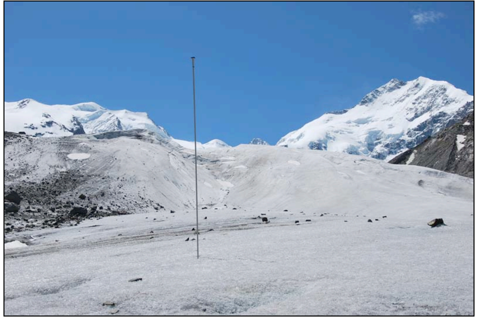
Ablation stake on the Vadret da Morteratsch, with a GPS receiver on top.
