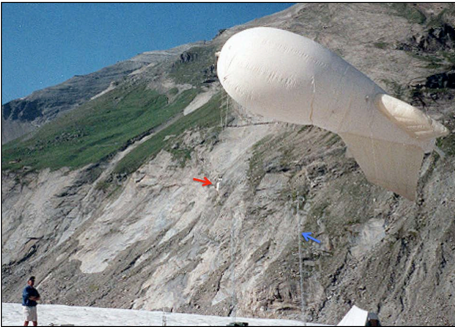
Figure 1.5. Operating a helium balloon of 11 m 3 on the Pasterzen Kees, Austria, summer 1994. The red arrow points to the sensor. A profile mast was used to probe the lower boundary layer (blue arrow). Photo made by Carleen Tijm-Reijmer.
