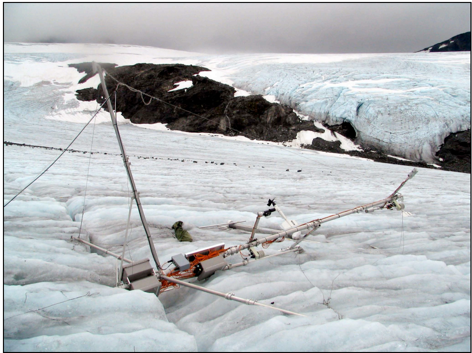
A crevasse damaged this AWS on Storbreen (photo by Liss Andreassen).
