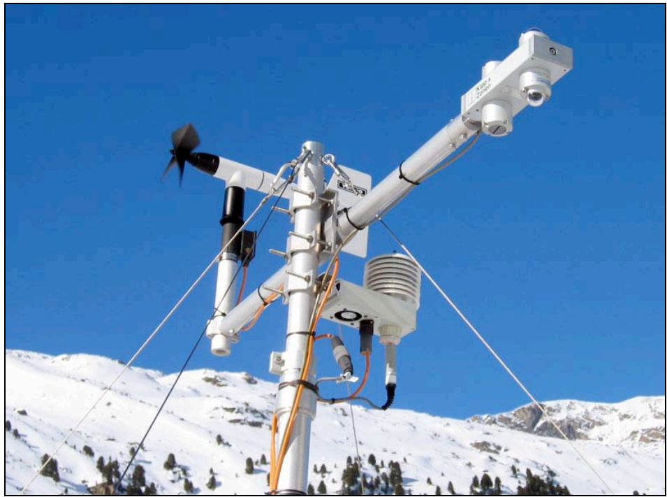
Sensors of the AWS on the Vadret da Morteratsch, October 2006.
