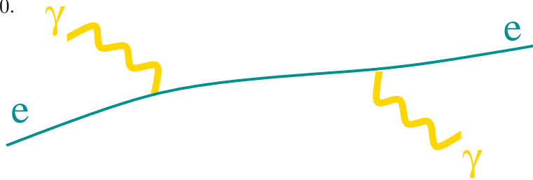
FIG. 61: A Compton scattering of a photon off an electron. A photon gets absorbed, and then reemitted at a different place. The strength of the interaction is given by the fine structure constant, \alpha_{\text{em}} \simeq 1/137 . If the emitted photon has a larger energy than the absorbed photon, the process is known as the inverse Compton scattering.
