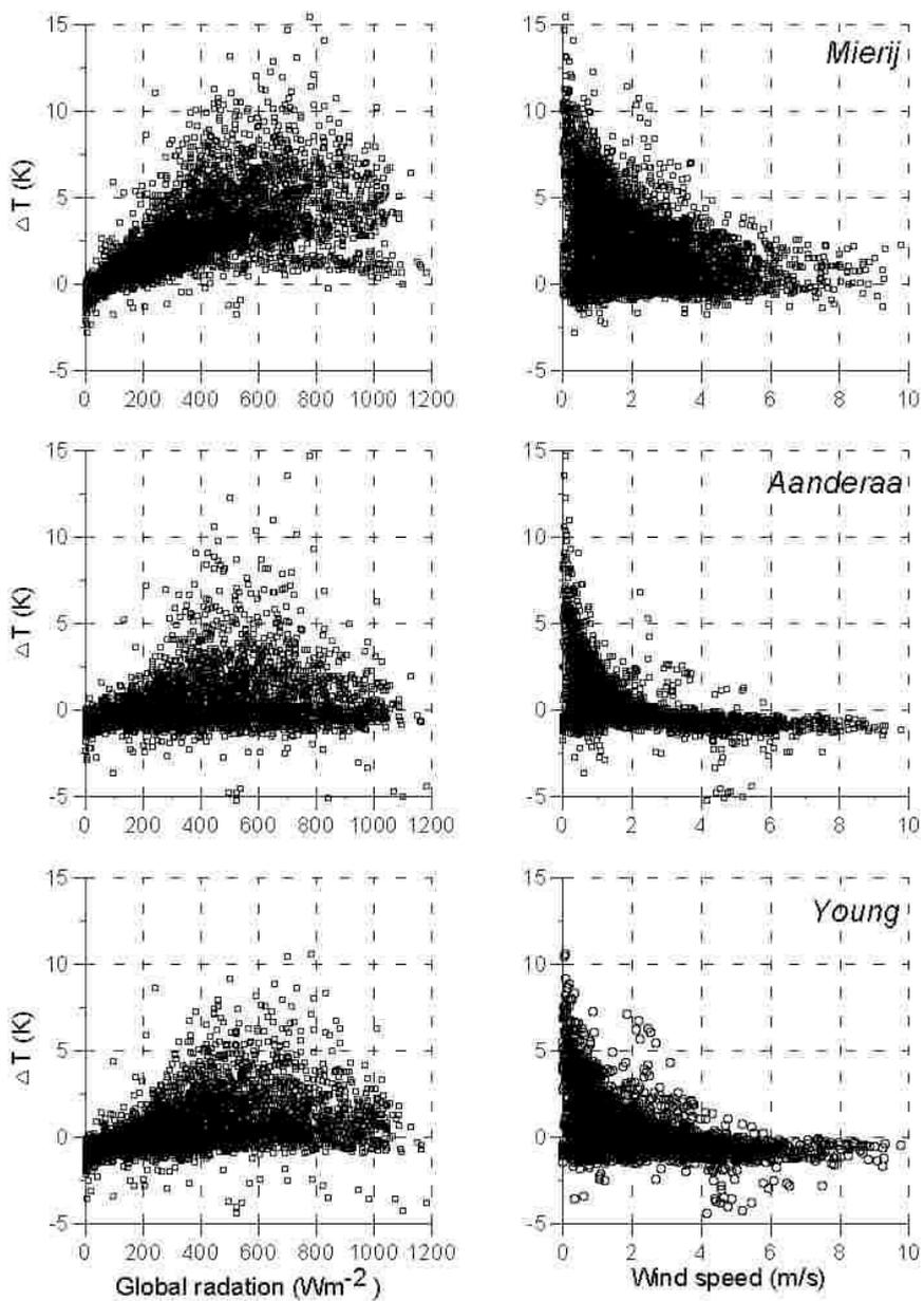
**Figure 3:** Differences between unventilated and ventilated air temperatures (10-minute averages) versus global radiation and wind speed.
