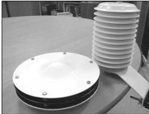
**Figure 4:** A Climetrics' screen beside a Young highlights the move away from an approximation to a Stephenson screen made by the three-plate design. The blackened internal plate surfaces reduce internal reflections whilst the metal plates provide improved thermal coupling.
