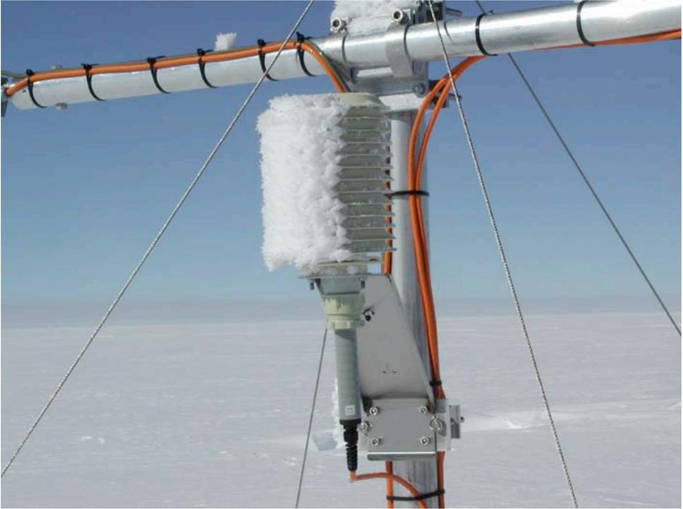
**Figure 3:** The Vaisala HMP35AC temperature and humidity sensor in a 10-plate Gill radiation screen at an AWS site in Dronning Maud Land, Antarctica (2892 m a.s.l.),(photo H. Oerter, AWI Bremerhaven).
