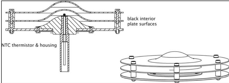
**Figure 3:** Unique temperature screen reduces radiation errors.
