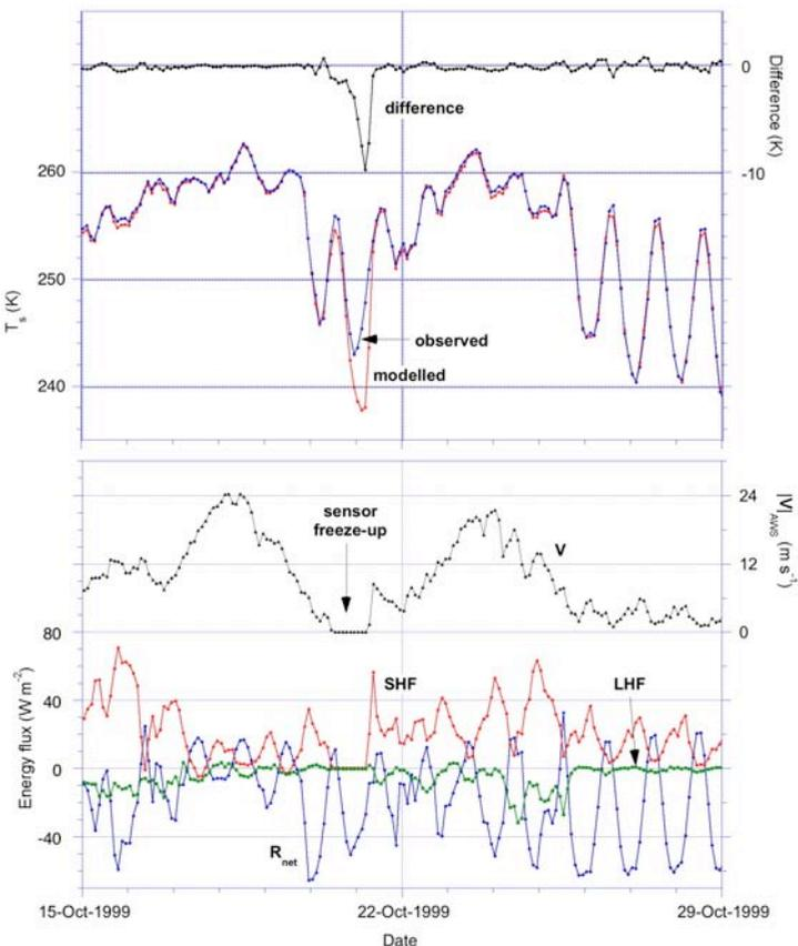
**Figure 3:** a) Modelled and measured surface temperature  $T_s$  and b) net radiation  $R_{net}$ , SHF and LHF at AWS 6 for a two week period surrounding a windspeed sensor freezing event.
