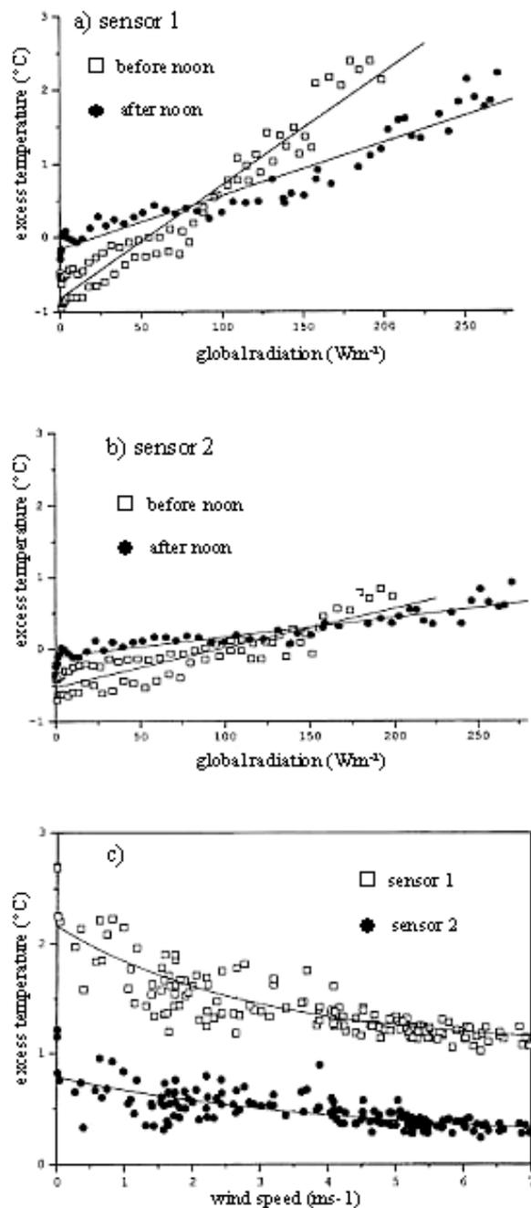
**Figure 2:** The effect of global radiation on the excess temperature of sensors inside of an original R.M. Young shield (sensor 1) and a R.M. Young shield with blackened down facing surfaces (sensor 2). The effect of wind speed on excess temperature measured within the two devices (relative to a standard Stevenson screen).
