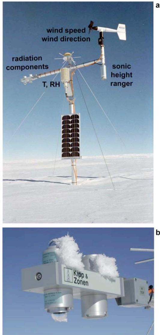
**Figure 2:** a) picture of AWS 9. The data logger and pressure sensor are buried in the snow; b) enlarged image of K&Z CNR1 radiation sensor.
