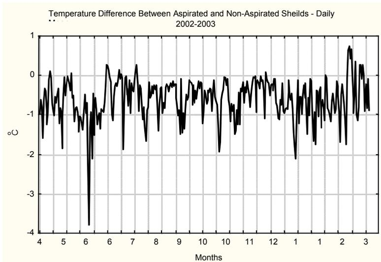
**Figure 4:** Mean daily temperature difference, ventilated vs. non-ventilated.
