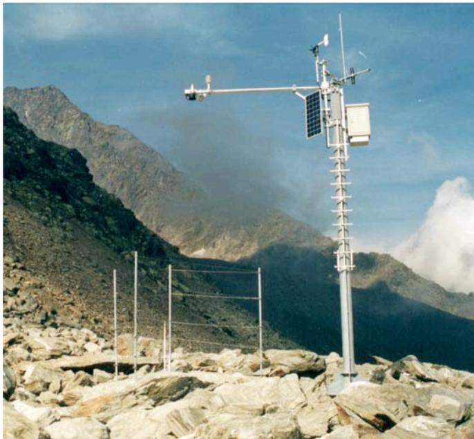
**Figure 1:** Automatic weather station for avalanche warning in the western Swiss Alps (Simplon Wenghorn, 2420m a.s.l.)
