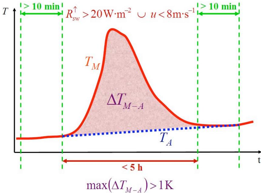
**Figure 3:** Automatic error detection used for extracting those measurements from the erroneous temperature time series that are a) susceptible to radiation errors, and b) for which the 'true' temperature values can be well approximated by linearly interpolating between the adjacent, undisturbed measurements. Detected errors, i.e., the differences between measured and interpolated air temperatures, are used for determination of the correction parameters by inverse modelling.
