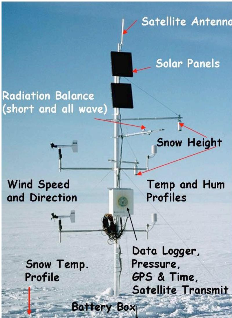
Figure 1: GC-Net automatic weather station instruments.
