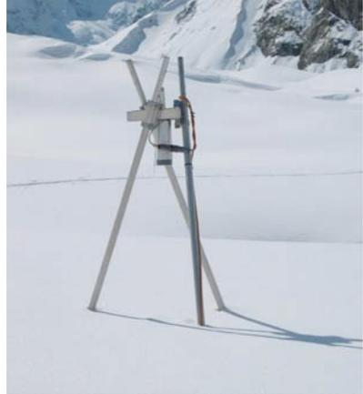
**Photo:** The sonic altimeter on the Morteratsch glacier. (Photo: Carleen Tijn-Reijmer)
