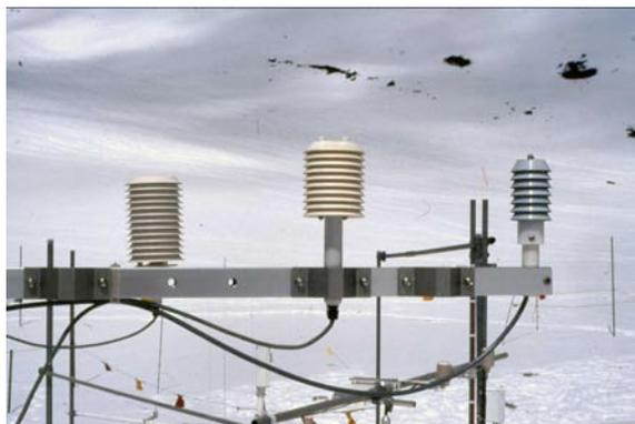
**Figure 1:** Radiation shields used in the experiment: Young (left), Mierij (middle), Aanderaa (right).
