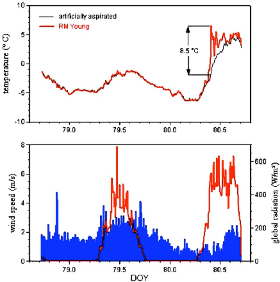
**Figure 1:** Measurements of temperature in an artificially aspirated (Kroneis 430M) and in a plate shielded (R.M. Young) device. The lower panel indicates wind speed and global radiation as measured at the site (Oberberg, 1999).
