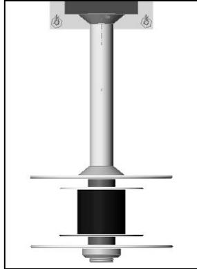
**Figure 6:** A pressure port designed to limit venturi errors. The parallel plates produce equal pressure changes in the internal cylindrical cavity. The pressure is vented to the transducer enclosure (top) from the midpoint of this cavity.
