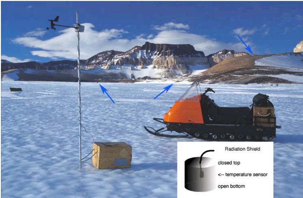
**Figure 2:** This picture shows one of the Davis weather stations in January 2003. The locations of three other stations are indicated by the arrows. The inset shows the design of the radiation shield used for the Davis temperature sensors.
