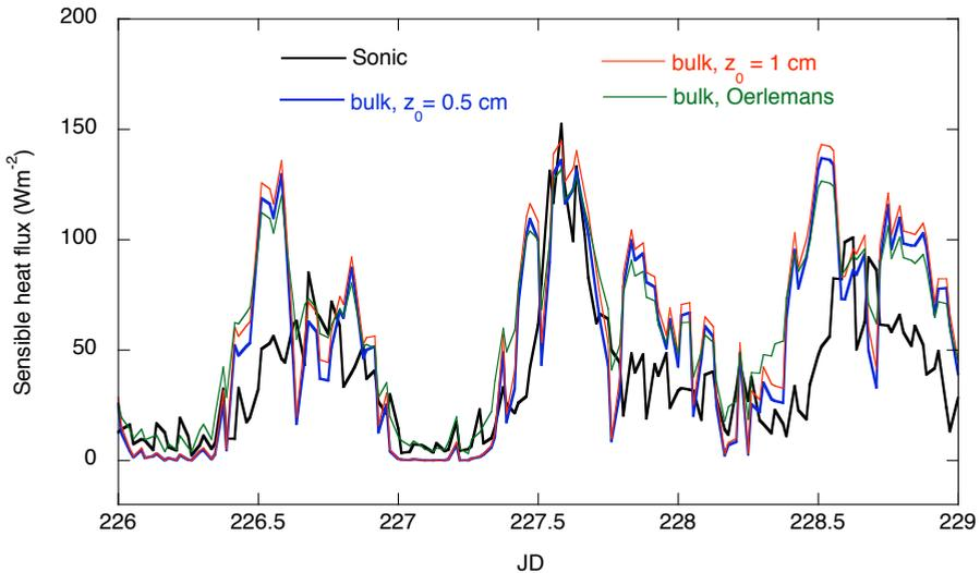
**Figure 3:** Sensible heat flux as measured by the sonic anemometer after tilt correction using the planar fit method, and calculated from the AWS using a bulk method and a constant turbulent exchange coefficient following Oerlemans (2000), and stability correction functions varying  $z_0$  between 0.5 and 1 cm. The data are for three summer days in 2002.
