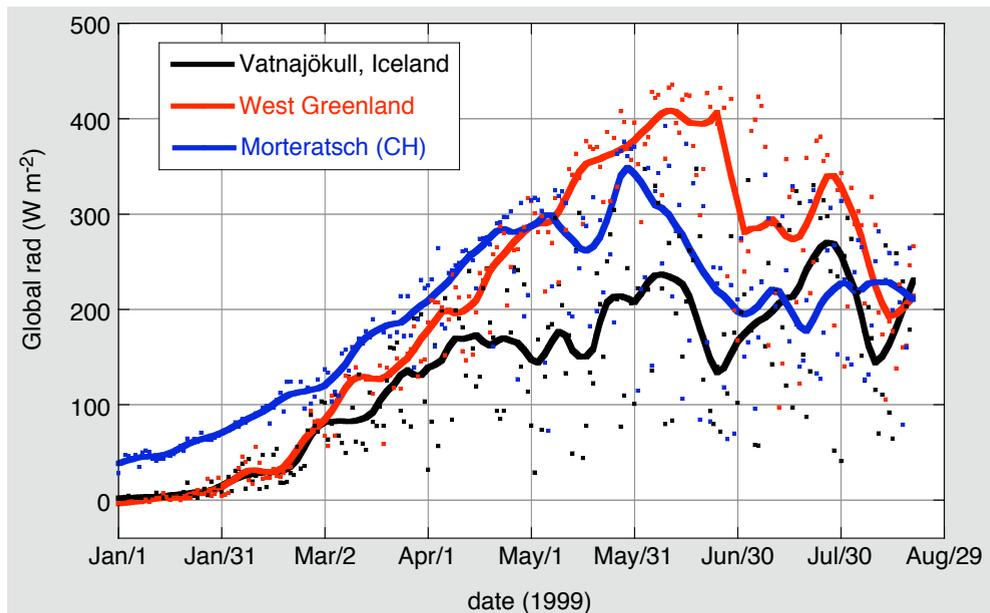
**Figure 3:** Daily mean values of global radiation at three different AWS sites. In the ablation zone of the ice sheet in West Greenland global radiation is about twice as large as on Breidamerkurjökull, Iceland.
