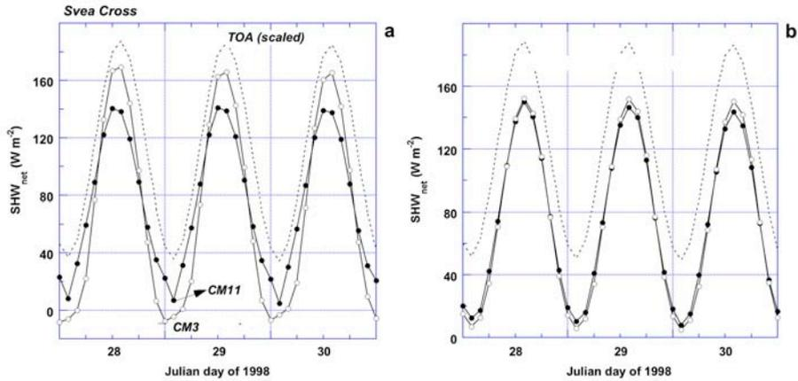
**Figure 3:** a)  $SHW_{net}$  for three days of fair weather at Svea Cross, as measured with the Kipp and Zonen (K&Z) CM3 and K&Z CM11.  $SHW_{\downarrow}$  at top-of-atmosphere (TOA) is also shown, scaled and offset for comparison; b) same as above, but after correction using the method of ‘accumulated albedo’.
