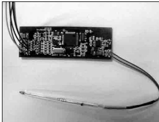
**Figure 2:** Precision temperature sensor interface and NTC thermistor. The intelligent sensor interface is used, with some transducer interface modifications, on all Climetrics' sensors.
