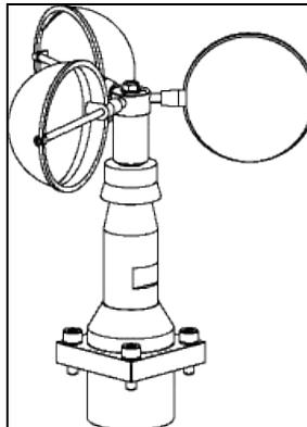
**Figure 5:** A custom anemometer design uses bearings that remain operational to  $-60\text{ }^{\circ}\text{C}$ .
