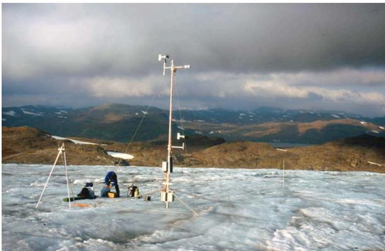
**Figure 2:** The IMAU-AWS on Hardangerjökulen, Norway, in September 2000 (photo by Wim Boot). The mast has four legs and stands freely on the ice. The mast is about 6 m high. Two sonic rangiers are used: one on a tripod drilled in the ice (8 m stakes), and one in the mast (below the Young anemometer).
