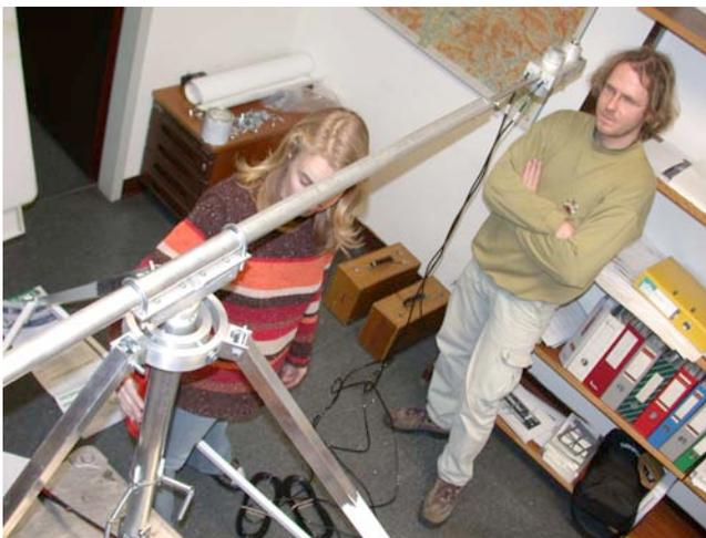
**Figure 2:** The cardan-like joint is the core of the self-adjusting mounting device (Foto: G. Kaser).
