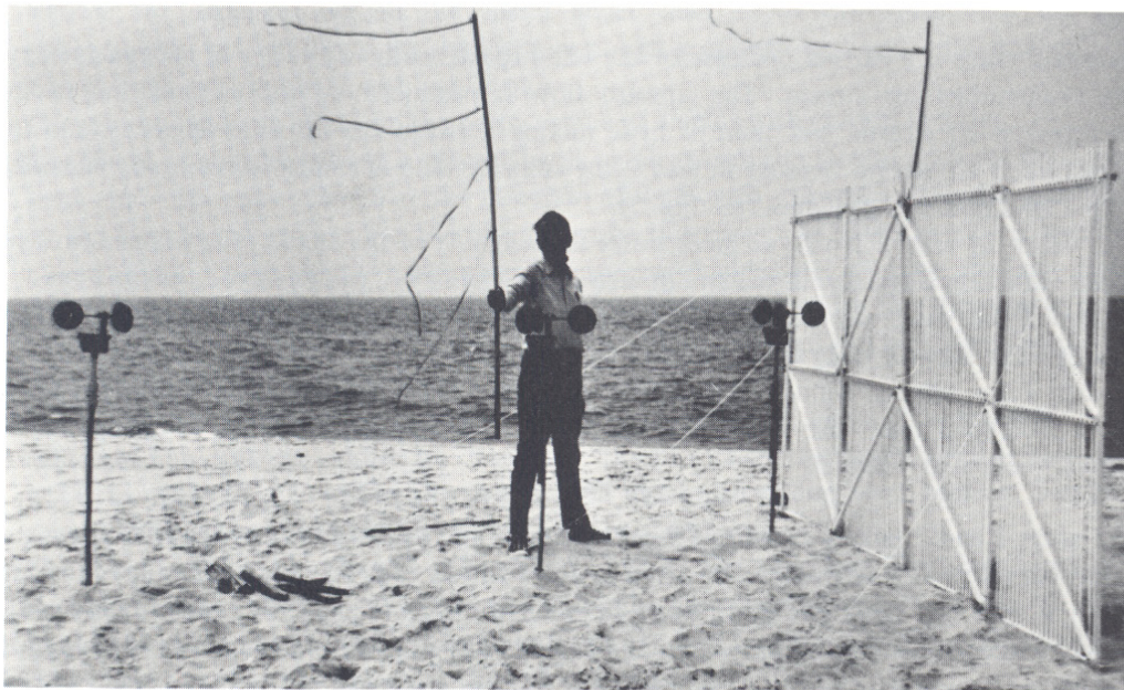
Fig. 5 the wind shields set up on the beach of Ilha da Barreta in South Portugal. The second and third ribbon on the rod show that the turbulent layer between the horizontally stratified air mass behind the shield and the undisturbed wind flow above the shield is very thin.
