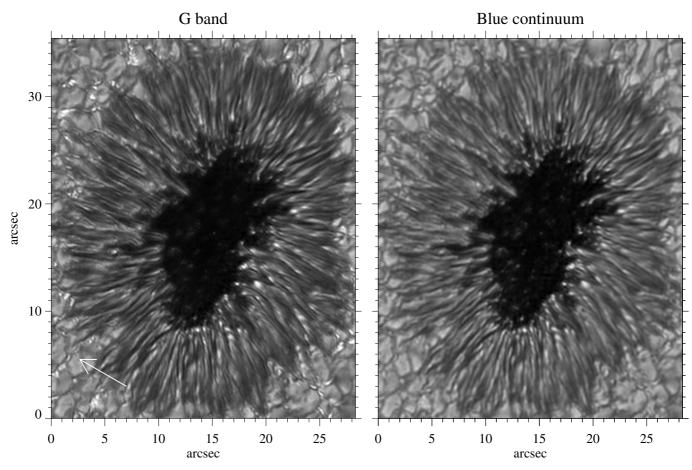
**Fig. 1.** Subfield of one of our best *G*-band (*left*) and blue continuum (*right*) filtergrams. The arrow marks the direction to disk center. The full field of view amounts to  $87 \times 70 \operatorname{arcsec}^2$ . The images are corrected for atmospheric distortions using the speckle masking method, and reach the theoretical resolution limit of the telescope of 0.2 arcsec.
