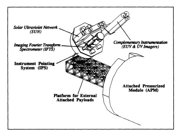
Fig. 1 — Possible implementation of the SIMURIS Model Payload at the far-end of the Attached Pressurized Module of the Space Station Freedom
