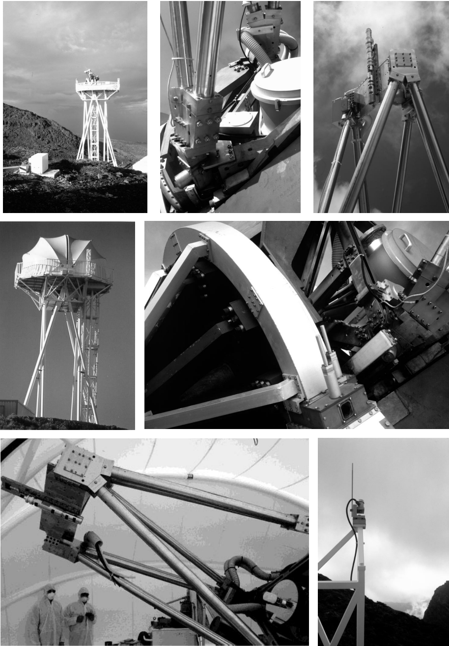
Figure 1. DOT photographs, along rows from top left: • DOT observing, water tank for prime-focus cooling in foreground. South is to the left. • covered mirror, focus support struts, suction hoses. • initial imaging-system tube. • clamshell canopy closed. • hour angle wheel, covered mirror in the upper right. • focus alignment within the canopy. • Seykora-Beckers scintillometer with anti-falcon spike.
