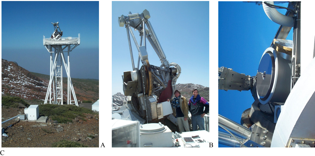
Fig. 2: a) The Dutch Open Telescope (DOT) on the La Palma, observing the sun; b) close up of the telescope; c) detail of the 45 cm primary mirror.
