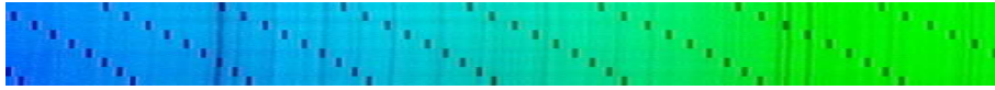
Figure 1. Tuning of barrier sub-filter transmitting spectrum maxima by its inclination. Each line represents the inclination of 1^\circ . As a result we can see tuning of the filter maxima. (Transmittance of the sub-filter is negative in this Fig.)
