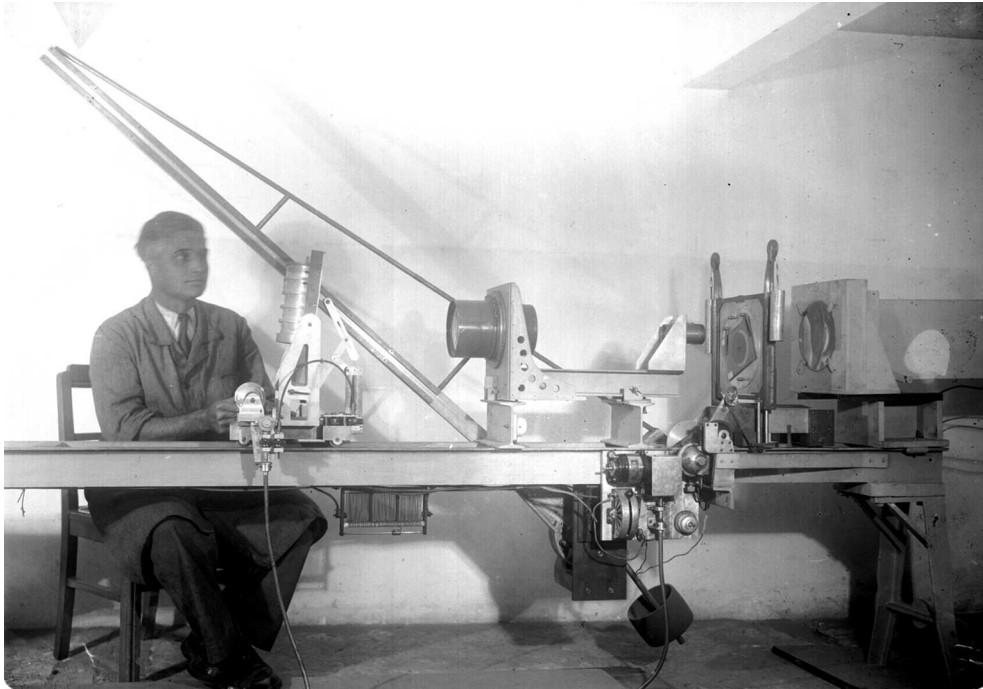
Figure 8. R. Servajean's optical anamorphoser with M. Brebion, the mechanic in charge of building the device.
