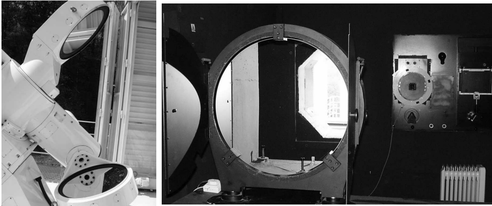
Figure 2. Left: The Jensch-type coelostat consisting of two 60 cm flat mirrors is located 4 – 6 m above the ground and is covered by a moving metallic shelter. Right: the main objective has a 50 cm parabolic mirror and 35 m focal length. To the right is the entrance slit of the spectrograph with the rectangular reflecting mirror for the slit-jaw system.
