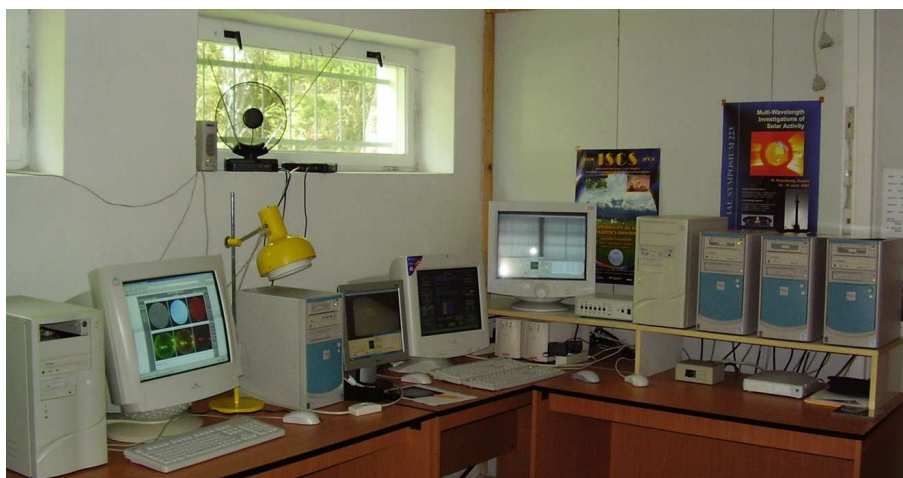
Figure 9. Before the reconstruction the observer controlled the spectrograph and telescope with a handbox near the entrance slit. Now his working place is a comfortable room in the basement of the pavilion to minimize man-made vibrations and heating.
