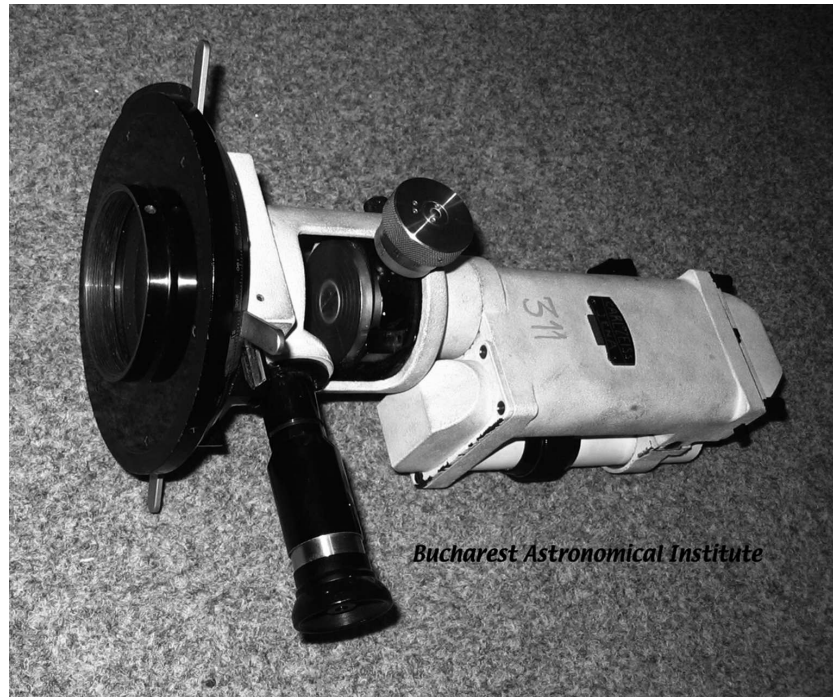
Figure 2. Janssen type spectroheliograph for prominence observation (courtesy Bucharest Observatory).
