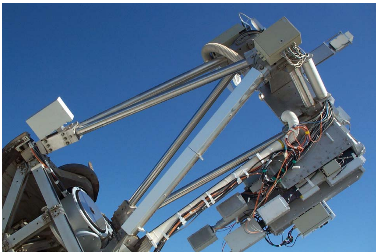
Figure 3. Barium and H \alpha filters at the Dutch Open Telescope. Left bottom: primary mirror. Right top: primary image. Right bottom: the H \alpha -filter box close to the telescope structure, underneath the Barium -filter box and, hanging on it, a small box of the new temperature controller. Inside the smaller boxes at the lower left side are the CCD cameras with fiber links for, from left to right, Barium, H \alpha , blue continuum near Ba and red continuum near H \alpha .
