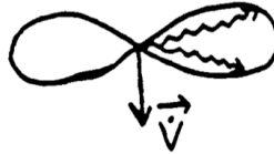
Figure 6.1: Dipole radiation from an accelerated charge.
