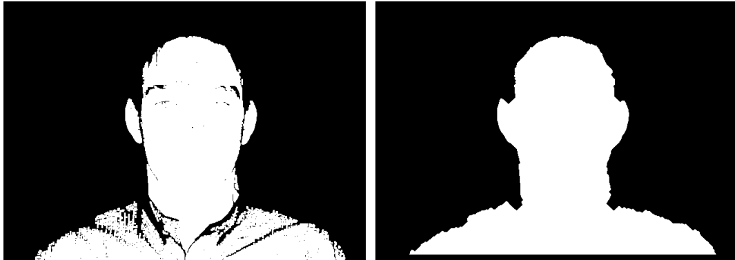
Figure 5.9. Closing and opening applied to the flag to eliminate gaps and irregularities.
