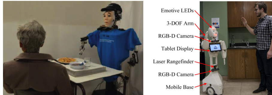
Figure 2 Left: Brian 2.1 socially assistive robot for the elderly and cognitively impaired (Source: [McCull et al. 2013]). Right: The Casper multimodal robotic kitchen helper. (Source: [Bovbel and Nejat 2014], Video at: https://youtu.be/noSJ9qWt_f0 )
