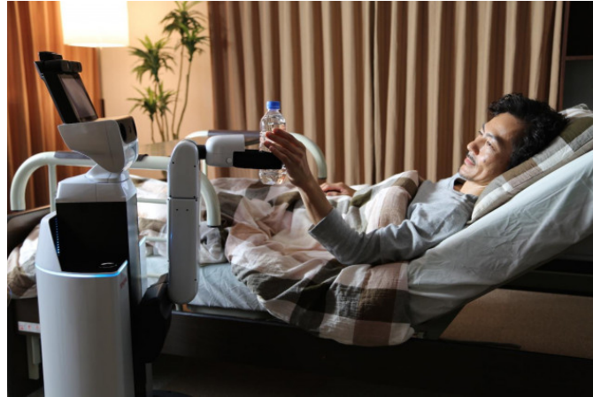
Figure 8 The Toyota Human Support Robot (HSR) system, planned to coexist with family members in a home environment. (Image source: [Kalogianni 2015], and video at: https://www.youtube.com/watch?v=QoS-40Xe75Q .)
